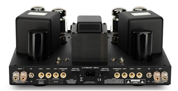
Similarly Spartan and logically distributed, the SLI-80HS's back panel includes two pairs of speaker binding posts, those toggle switches for choosing 4 or 8 ohm taps from the output transformers, three RCA inputs marked Line 1, 2, and 3, RCA subwoofer outputs, a fuse holder for each channel, and an IEC connector receptacle.
